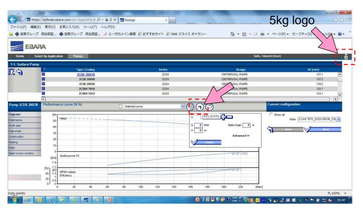
Input required duty point Q, H, and static head. Then click "apply".
