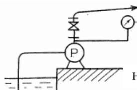
Gauge pressure at valve full-open is the pressure (head) actually required at site.
